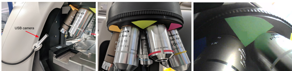
Figure S1: Close-up of the objective detection mechanism: A USB camera is pointed at the nose piece ring for detection of color coded markers that are unique for each objective ring position.
